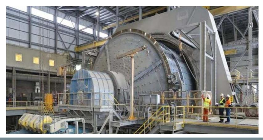
SAG Mills Are Used In Large Mining Operations To Grind Crushed Ore Prior To Processing To Recover Valuable Metals
